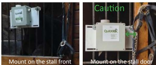
The system may be mounted on either the stall front or the stall door.
